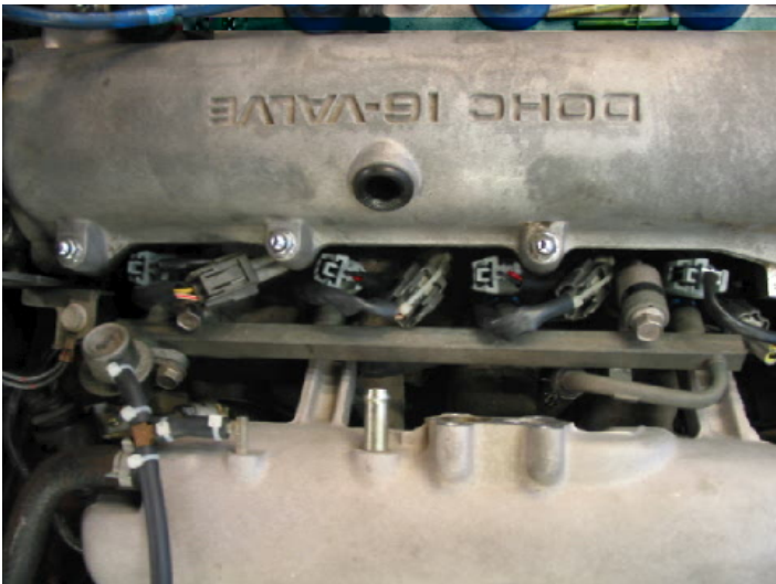
Figure 27: Fuel injector installation
