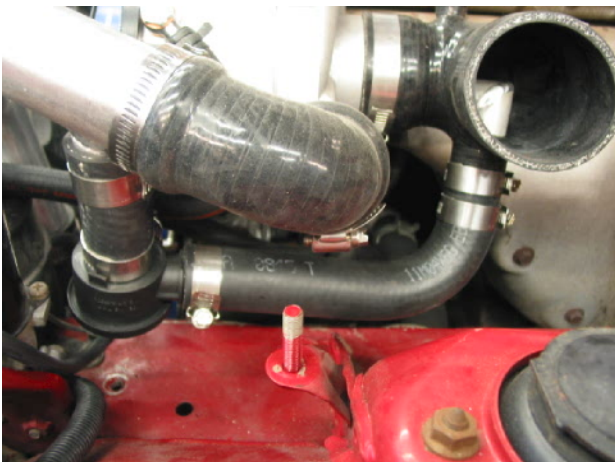
Figure 18: Bypass valve installation
